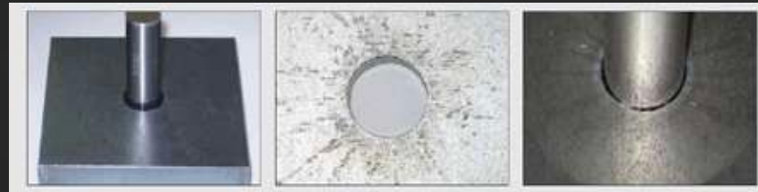
12 mm hole with True Hole Technology cut with HPRXD Plasma.
